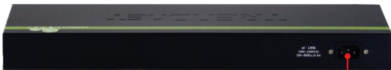
1. Connect the **Power Cord** to the TE100-S16g/TE100-S24g and then to a power outlet.
