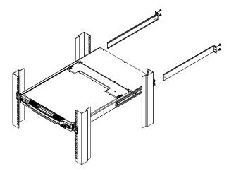
3. After the L brackets have been secured, tighten the front bracket screws.
