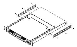
2. Attach the left and right *easy-installation* mounting rails to the inside of the rack. The flange that supports the switch will be to the inside.
